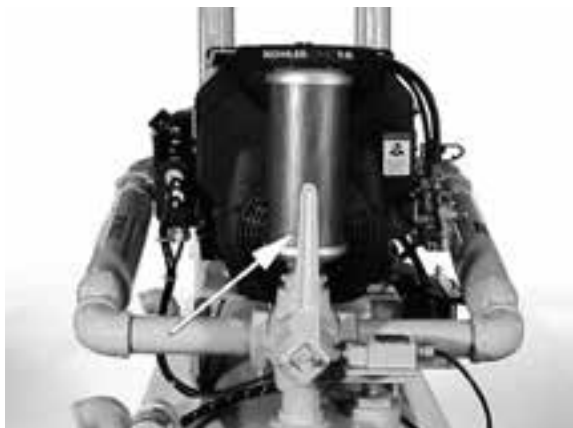
FIGURE II-B Suction/Discharge lever - DISCHARGE position
