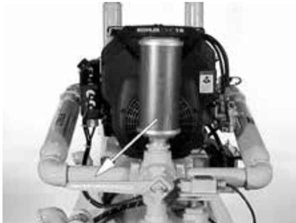
FIGURE II-A Suction/Discharge lever - SUCTION position
