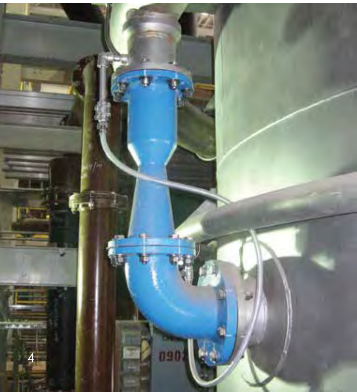
Improvement in sulfide recovery using the Cavitation-Tube sparging system when treating -50 micron fines.
