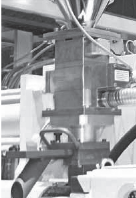
Model CFP Metal Separator at the material infeed throat of an injection molding machine
