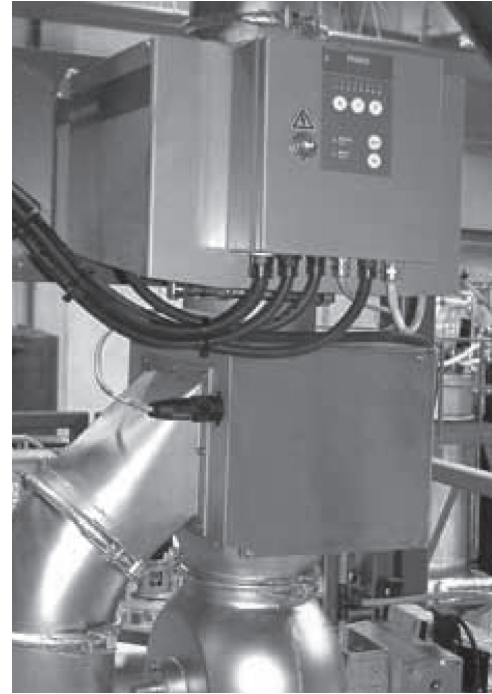
Model FF Metal Separator used for the quality control of PET regrind
