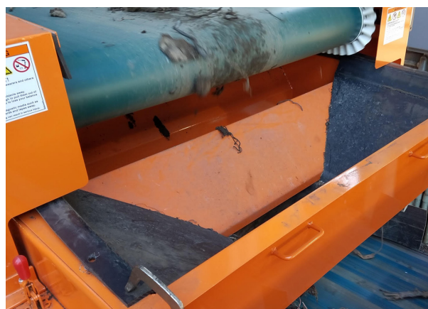
Equipment utilized within the Zurik to Zorba process consists of a ring mill, small drum type magnetic separator, high frequency eddy current separator and a stainless steel magnetic separator.
