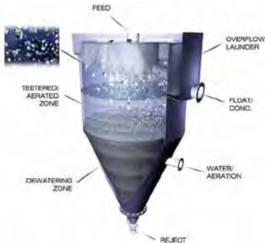
FIGURE 3 Simplified diagram of the HydroFloat® cell
