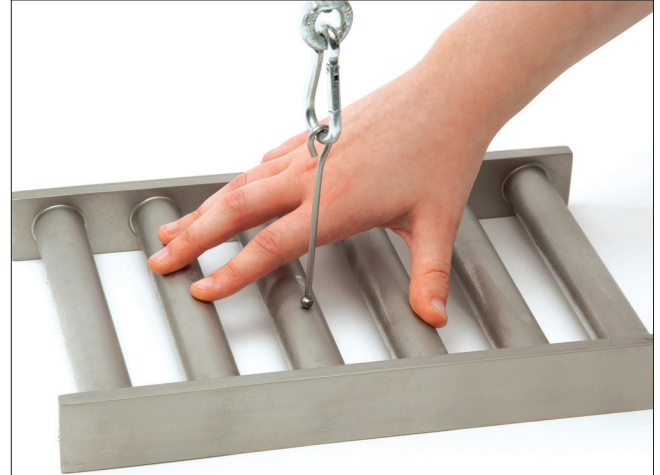
Rare Earth Grate Magnet Pull Test using a 1/4" ball (6mm) test piece.
