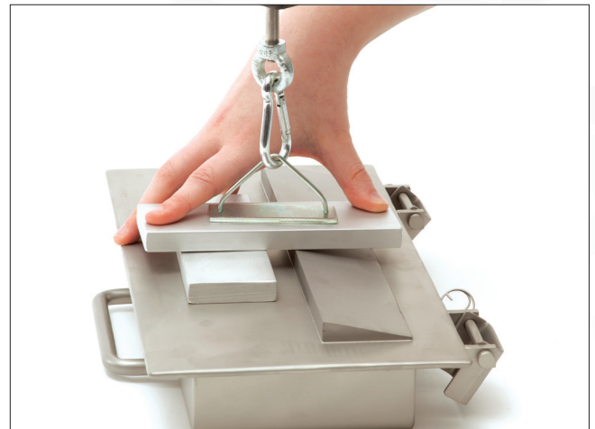
Rare Earth Plate Magnet Pull Test using non-magnetic spacers & 1/8" bar (3mm) test piece.
