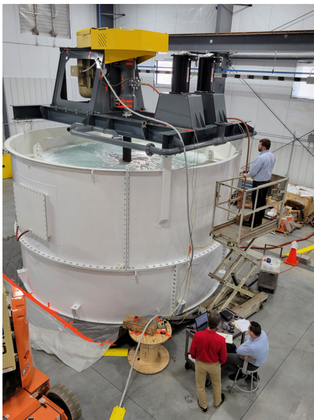
Figure 5. Eriez engineers performing hydrodynamic tests on a StackCell SC200.
