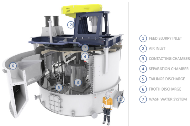
Figure 4. Cutaway of the 2-stage Eriez StackCell®.
