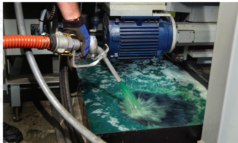
Once filtered, coolant is returned to the sump at a rate of 20 to 40 GPM.
