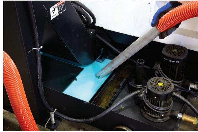
Machine tool coolant, chips and sludge are easily vacuumed out of the sump.
