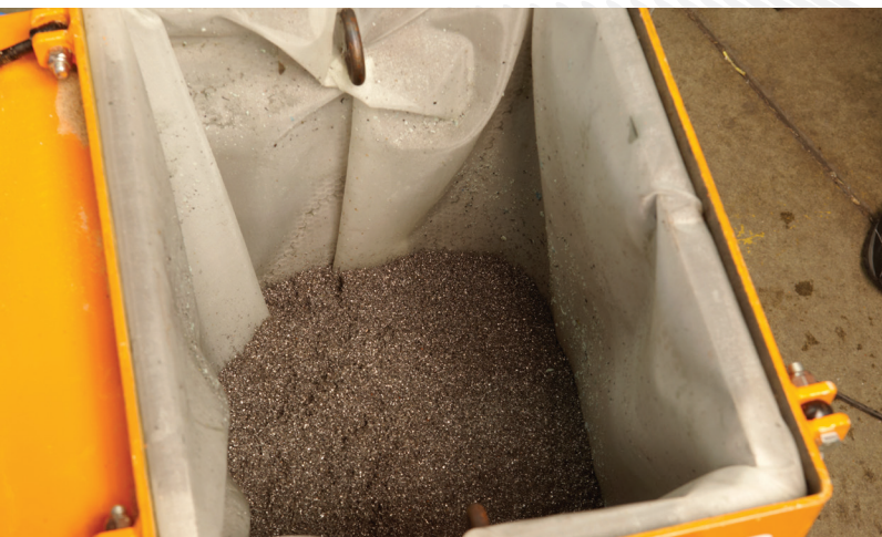
The reusable polypropylene filter sleeve is inserted into the chip basket to filter coolant to 50 microns. Finer filtration of 20 microns nominal can be achieved with a single use paper filter sleeve.
