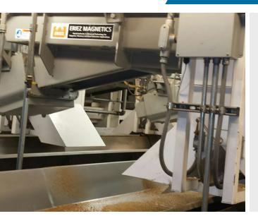
Heavy Duty Eriez<sup>®</sup> Vibratory Feeders Ensure Constant Pre-Crushed Sandstone Flow at Edwards Sand & Gravel
