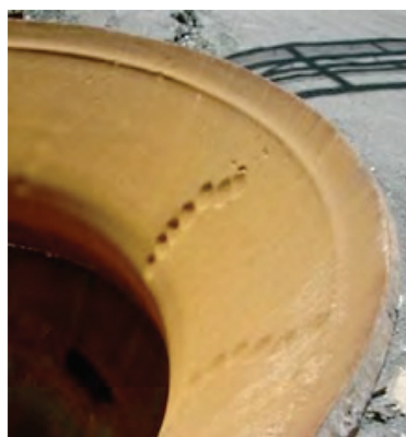
Figure 1: Cone crusher mantle damaged by a grinding ball
