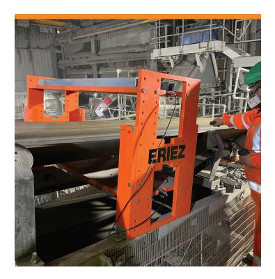
The latest MetAlarm marks a leap forward in signal processing and electronic design, using pulse-induction technology and adaptive digital electronics. Designed to maximize metal recovery during the inspection process in harsh environments like quarries, enhancing protection for crushers, screens, and conveyor belts by reliably detecting damaging tramp metal.
