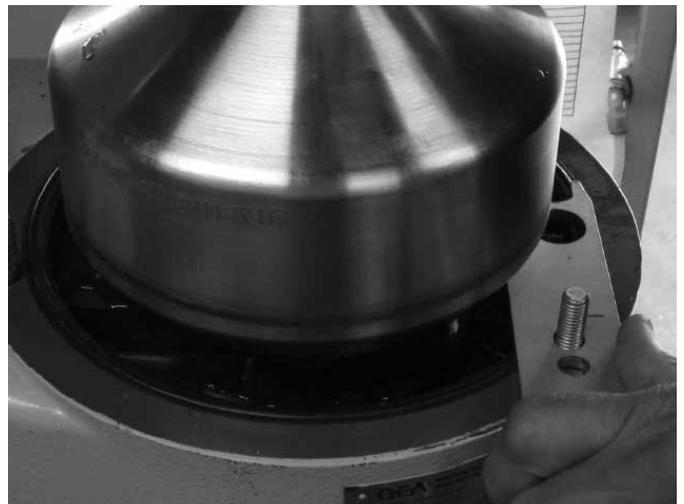
7. Place ring dam in the center of the pump chamber. It cannot be touching the inside of the pump chamber.
