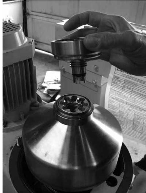
11. Place your thumbs of both hands on separating disc where it sits above the bowl top. With the other fingers on the bottom of the bowl top, press down with your thumbs while lifting with your fingers. Lift the bowl top straight up and off.
