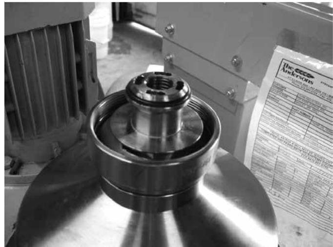
8. Place one wrench over the stud in the frame and place the hook on the wrench into the slot on the bowl bottom.
