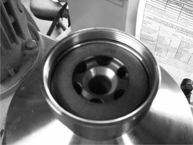
8. Place centripetal pump into the chamber.
