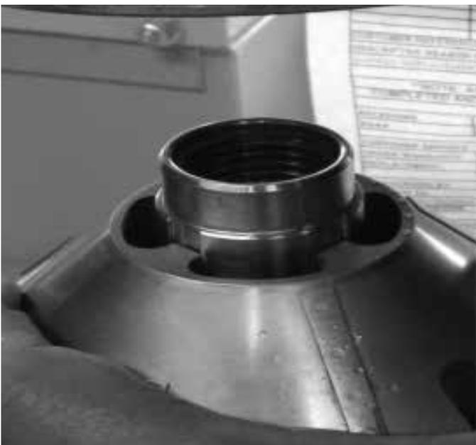
3. The separating disc top should sit directly on top of the disc stack with no gap.
