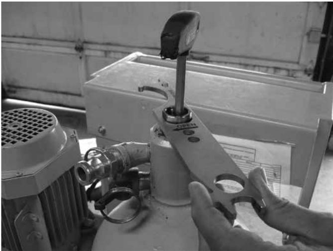
4. Remove the handle connection piece by pulling it straight up. Inspect the o-rings on it.
