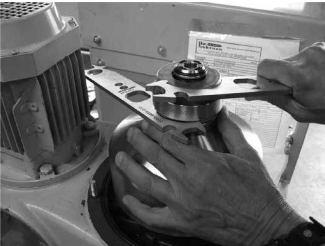
10. There should be no threads showing on the centripetal pump cover if assembled correctly.
