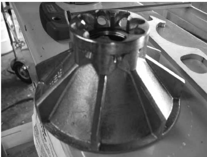
13. Holding the bowl top in one hand or placing on a bench, use a thin screwdriver to gently pry the loose end of the sludge liner away from the bowl top.
