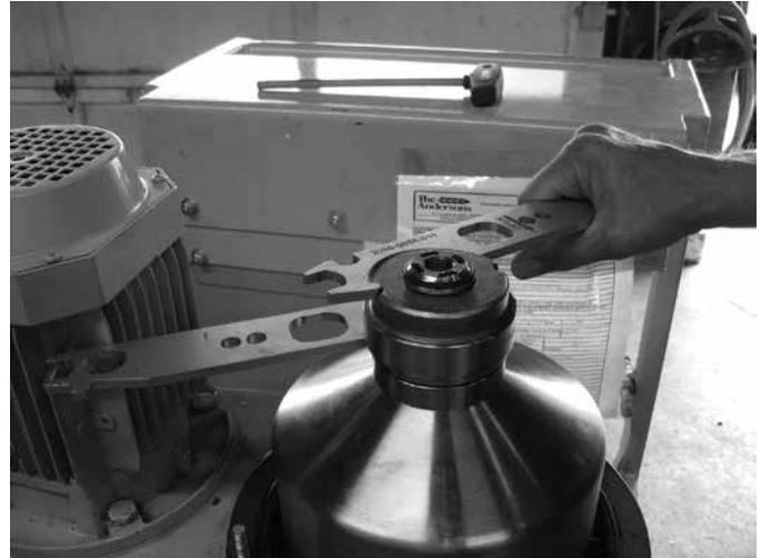
7. Remove the centripetal pump, inspect the gaskets. Remove the ring dam.
