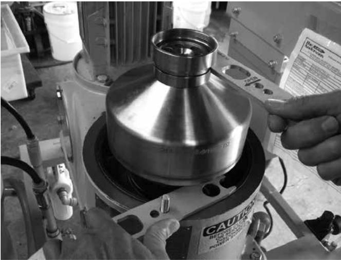
10. Remove the chamber and inspect the gaskets.
