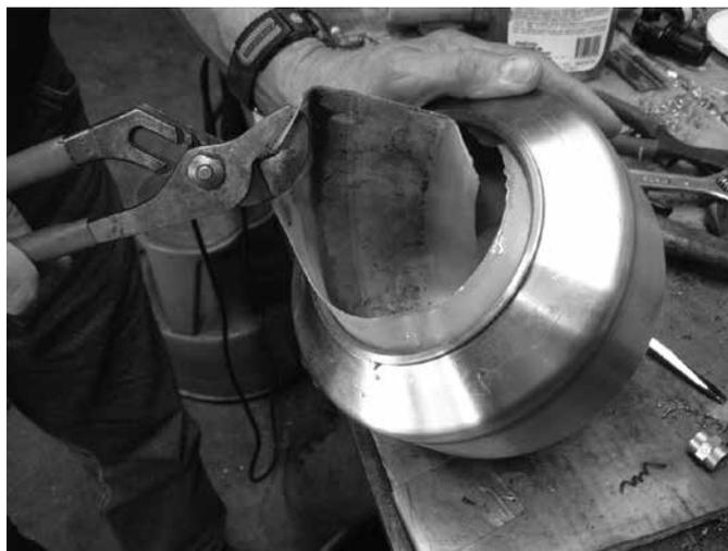
15. Clean the liner. The liner can be reused many times until it breaks apart.
