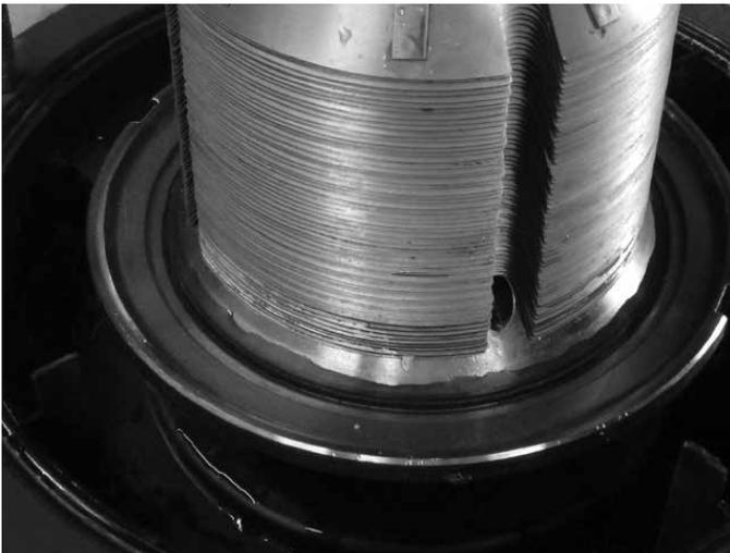
2. Make sure the o-ring on the inside of the separating disc is in place and put on the distributor/spindle over the discs while pressing down on the disc stack.
