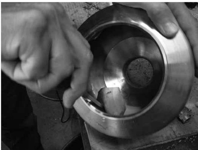
14. Take pliers and pull on the loose end of the liner and pull it out of the bowl top.
