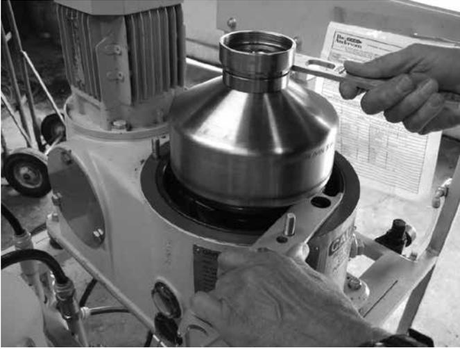
9. Place second wrench with its hook in the slot on the bottom of the centripetal pump chamber and turn clockwise (open).
