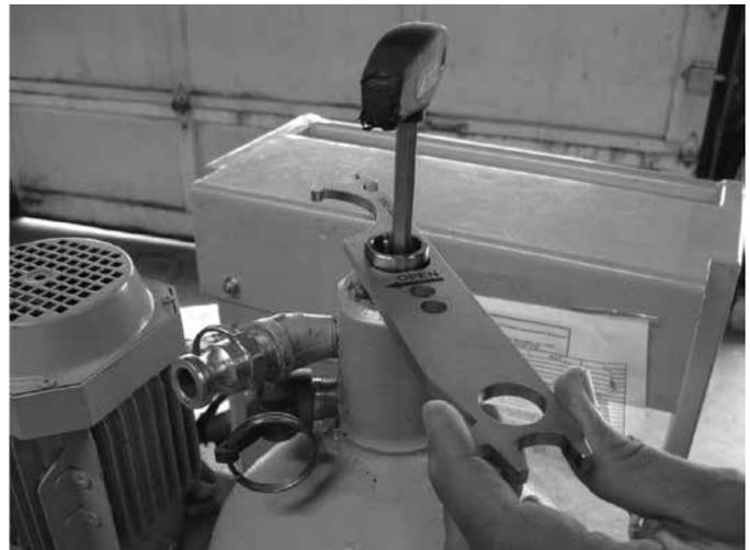
15. Screw the screw plug into the hood until snug. **DO NOT OVERTIGHTEN!**
