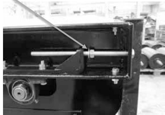
Ensure nuts & bolts are tight
