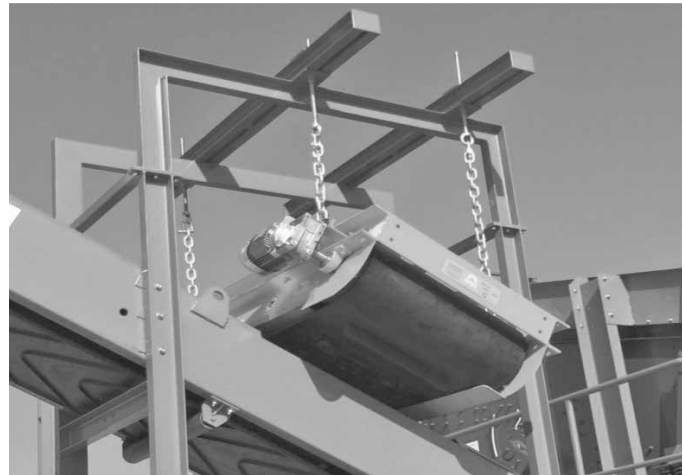
Typical Installation (chains not included)
