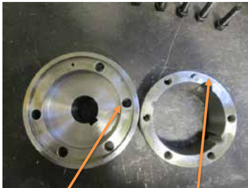
Recess to help assembly of both coupling halves
