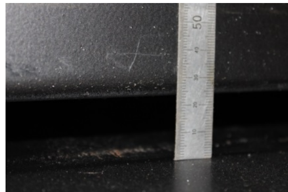
FIGURE 8 Typical Belt Sag 25mm (1 inch)
