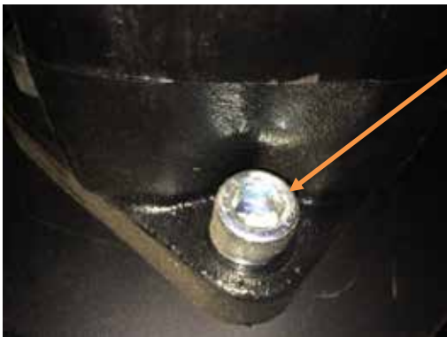
Recess to help assembly of both coupling halves
