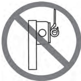
Avoid placing the magnet in shear.
