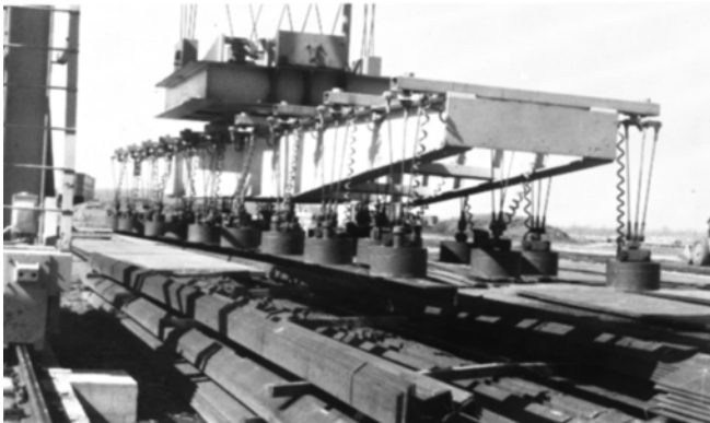
Multiple Selecto electromagnets on a lift beam.
