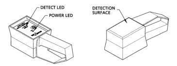
The sensing area of the detector is located in the base of the unit directly below the DETECT LED. You can determine the effective size of the detection area for your set of circumstances by turning the detector on and checking on the base (flat) side of the unit for the area of response.
