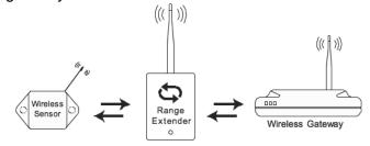
If the sensor detects a stronger signal from the range extender, it will automatically connect to the range extender.
