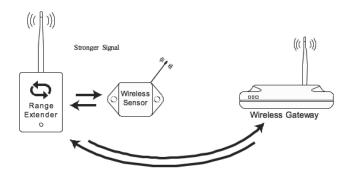
If the sensor detects a stronger signal from the gateway, it will automatically connect to the gateway and ignore the range extender.
