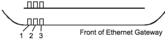
**Light 1** - Indicates the Ethernet cable is plugged in. A green light indicates ready and working, a red light indicates there is a problem.
