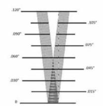
Deflection sticker showing .060" of total deflection. Each unbroken horizontal line above that zero line represents .015" of total deflection. Numerical scale will actually be blurred.
