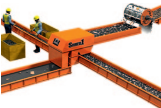
Eriez goal in developing its CleanStream Technology and Shred1 Separator was to produce No 1 Shred at less than 0.17% of greater copper content in the steel from a 100% vehicle feedstock.
