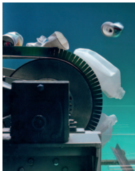
Eriez' eddy current separator in action.
