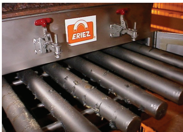
Iron particles are held against the magnetic tubes.
