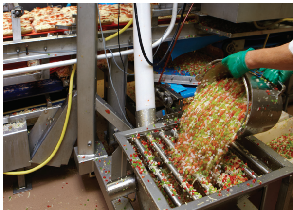
Magnetic grates allow free flowing product to pass between the magnetic tubes.
