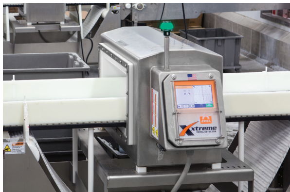
Metal detectors are used for raw material and finished goods inspection.
