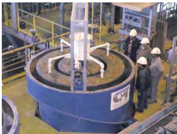
FIGURE 1 Typical industrial column flotation cell
