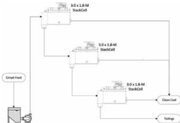
FIGURE 4 Generalized flow sheet for Patriot Coal's Kanawha Eagle floatation circuit
