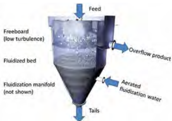
FIGURE 4 A cut-away of the Eriez HydroFloat® fluidized bed flotation machine
