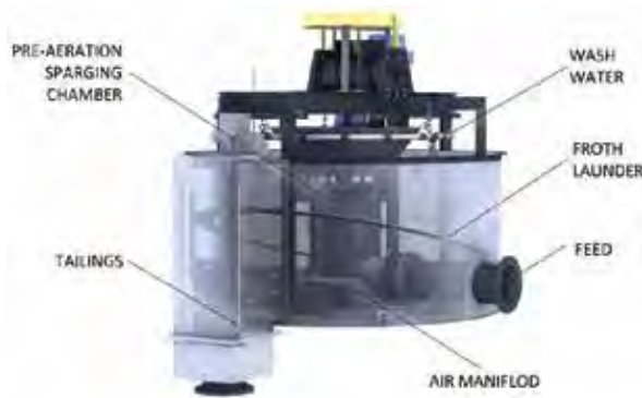
FIGURE 1 Schematic of the Eriez StackCell™
