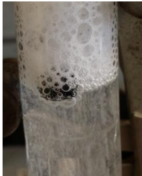
Figure 4 – Coarse particle trapped below the froth phase in a micro-flotation cell due to inadequate buoyancy of the particle-bubble cluster.
